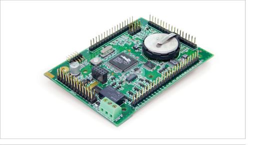
The LP3500 is a low-power single-board computer designed to operate reliably in any place it is deployed, especially where power is limited, such as in portable, hand-held, battery-powered, remote monitoring systems. The LP3500 features built-in analog and digital I/O, while consuming less than 20 mA when fully operational and less than 100  $\mu$ A in power-save mode.
